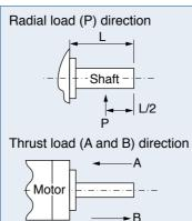
Because the radial load and thrust load significantly affect the life of the bearing, take care not to allow the load during operation to exceed the permissible radial load and thrust load shown in the table below.
